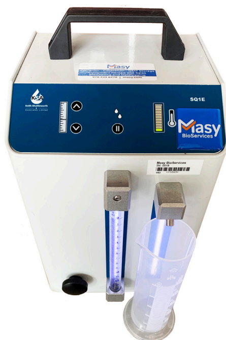
Figure 1: Non-Condensable Gas Test kit. Setup includes condensing unit and 250mL measuring cylinder.
