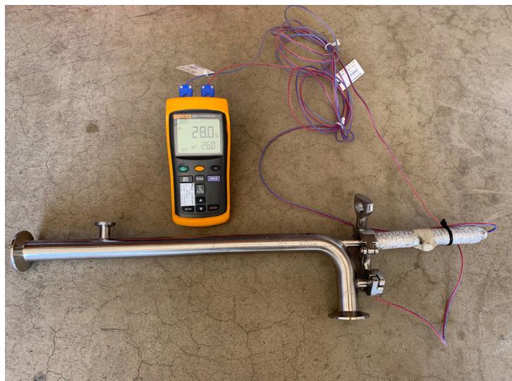
Figure 2: Superheat test kit. Setup includes sample port pipe, pitot tube, superheat expansion tube and temperature probes.
