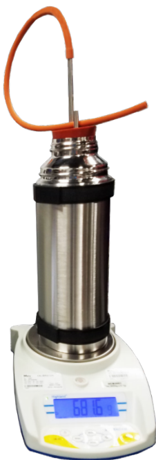
Figure 3: The Dryness Test Kit consists of a scale, steam supply tubing and an insulated flask.
